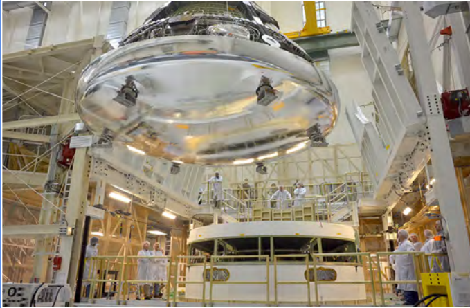
Orion's crew module is maneuvered into place above its service module in the Operations and Checkout Facility at NASA's Kennedy Space Center in Florida.
