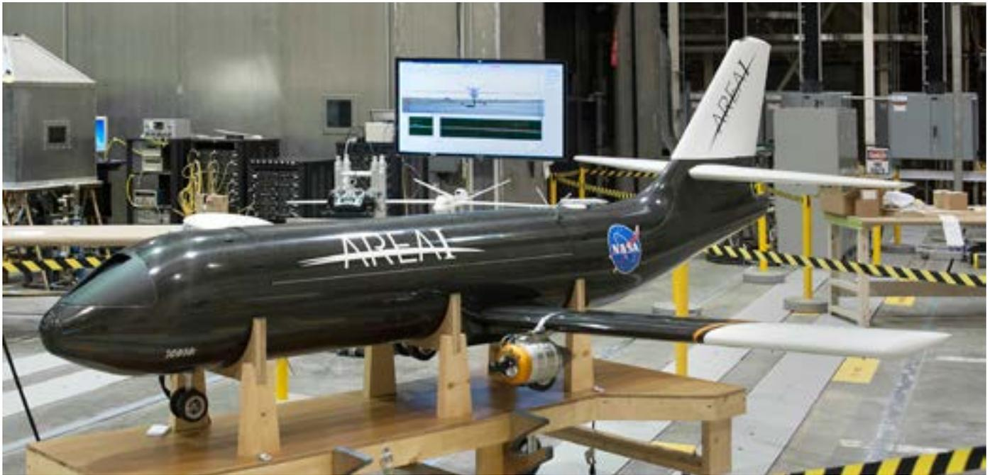
Seen here in the Armstrong Flight Loads Laboratory, the semi-modular PTERA may be reconfigured to accommodate a wide variety of flight experiments. (NASA photo/Ken Ulbich)
