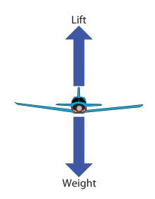
Fig. 6 Forces of straight and level flight
