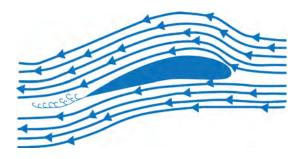
Fig. 3 Air approaching and passing over the surface.
