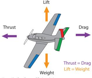
Fig. 9 The four forces of flight in balance
