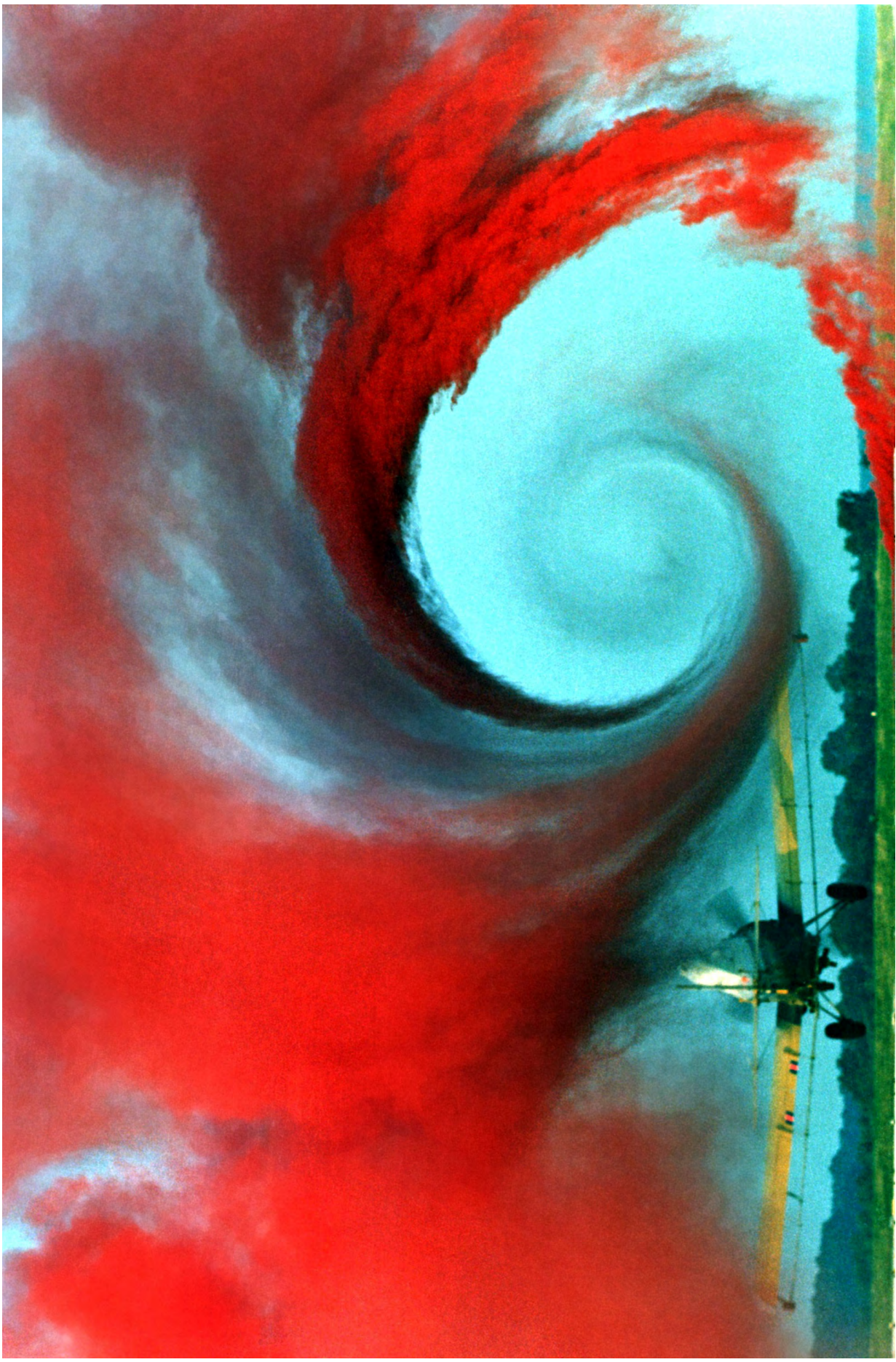
Img. 6 A wake vortex study at Wallops Island, VA
