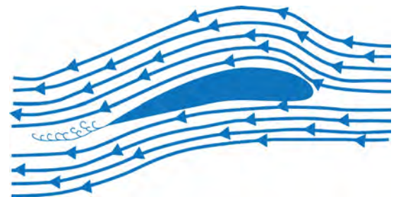
Fig. 3 Air approaching and passing over the surface.
