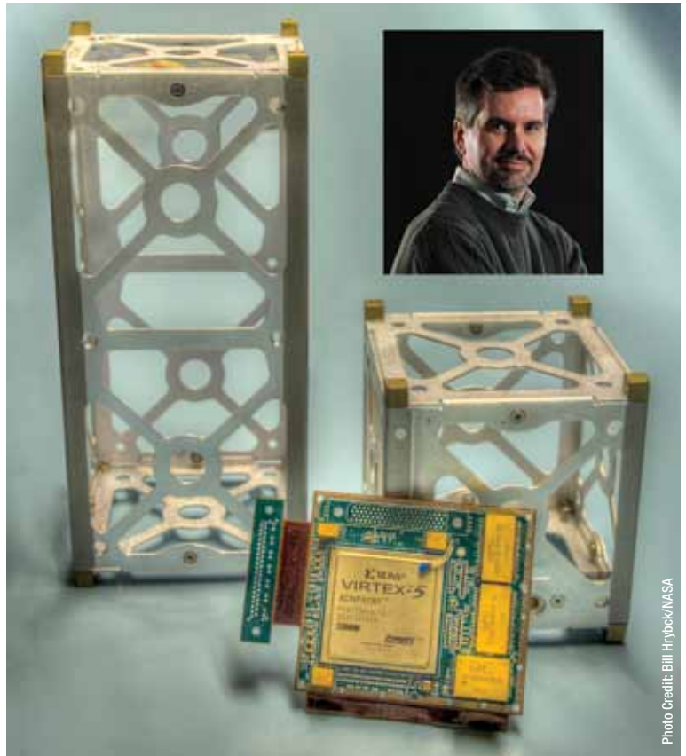
This year's winner of Goddard's "IRAD Innovator of the Year" award, Tom Flatley (inset), has played a pivotal role advancing the SpaceCube family of products. Shown here is the SpaceCube-Mini, along with two other devices that show the relative sizes of tiny satellites or Cubesats on which SpaceCube is slated to fly in the future.
