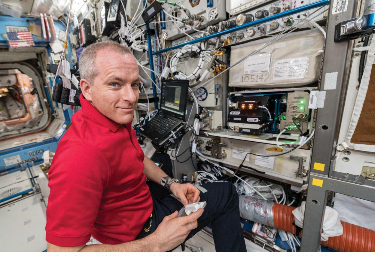
Flight Engineer David Saint-Jacques conducts field calibration operations for the Bone Densitometer Validation experiment. Densitometry measures the mass per unit volume (density) of minerals in bone, which is key to the development of countermeasures for human crew members aboard the space station, as well as for bone loss syndromes on Earth.
