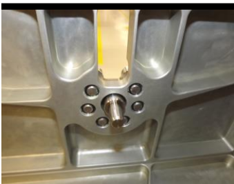
(INTERNAL VIEWS OF “TUNING FORK” AND SIX BOLT HUB MOUNTING PINS)
