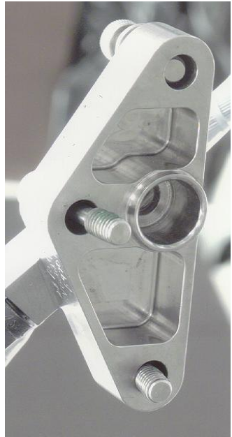
O2 FILL LINE HOUSING
