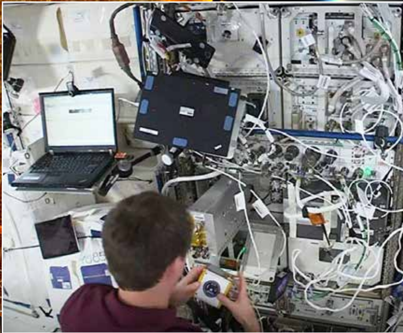
ISS installation of the MSU Computer by ESA astronaut, Thomas Pesquet (bottom = Pesquet taking computer out of storage bag; top = Pesquet plugging the computer into the NanoRacks internal experiment locker).
