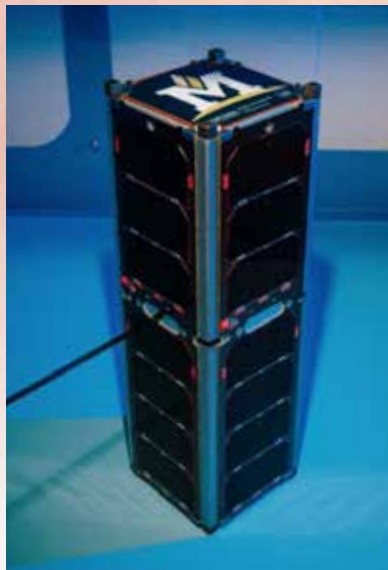
RadSat-g from Montana State University tests a new computer architecture that can recover from faults caused by space
