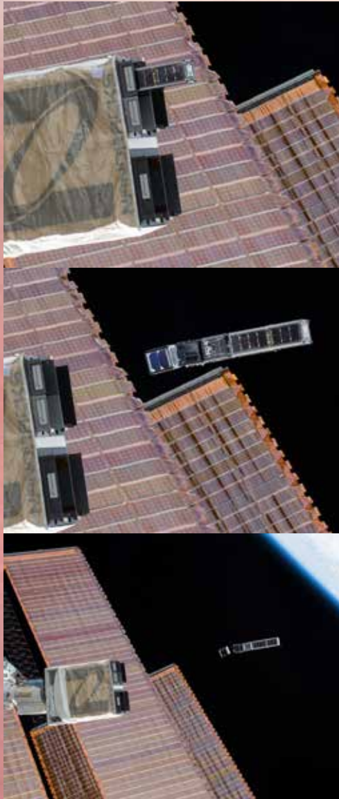
RadSat-g being deployed out of Deployer from International Space Station
