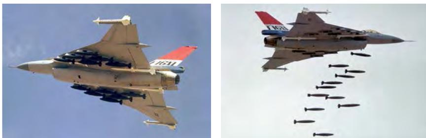
On left: The F-16XL-1 flying a test mission on August 18, 1982, with 12 500-pound Mk-82 bombs, 4 fuselage-mounted AIM-120 AMRAAMs, and 2 wingtip-mounted AIM-9 Sidewinder missiles. On right: On August 24, 1982, the F-16XL-1 successfully released 12 500 pound Mk-82 bombs from individual low-drag ejector bomb racks. (Both images USAF)
