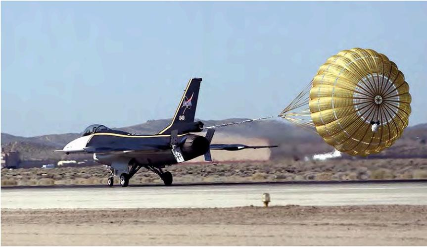
F-16XL-1 is seen during landing rollout with its drag chute deployed and the speed brakes on either side of the engine nozzle in the open position. (NASA)
