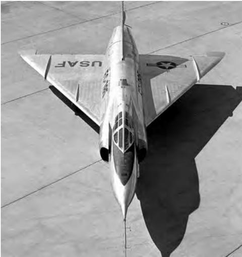
A Convair YF-102 Delta Dagger, flown by NACA at Edwards in 1954 on drag and aerodynamic pitch-up studies. (NASA)
