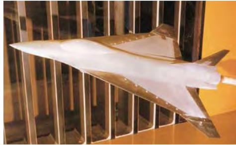
SCAMP matrix model seen during 1978 tests in the NASA Langley Unitary Plan Wind Tunnel. (NASA)
