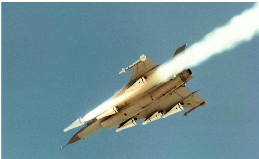
An unguided AGM-65 Maverick missile was launched from F-16XL-1 store station 3 on March 29, 1985. Weapons carried on this flight included four dummy AIM-120s, two AIM-9Ls, and six AGM-65 missiles. (USAF)
