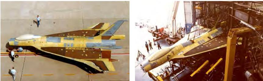
On left: The first F-16XL, 75-0749, is seen in April 1982 after its removal from its assembly fixture. The composite wing skins and wing-fuselage mounting bolt locations are evident. On right: The F-16XL-1 is seen being prepared for static structural proof testing in the spring of 1982. (Both images Lockheed Martin)
