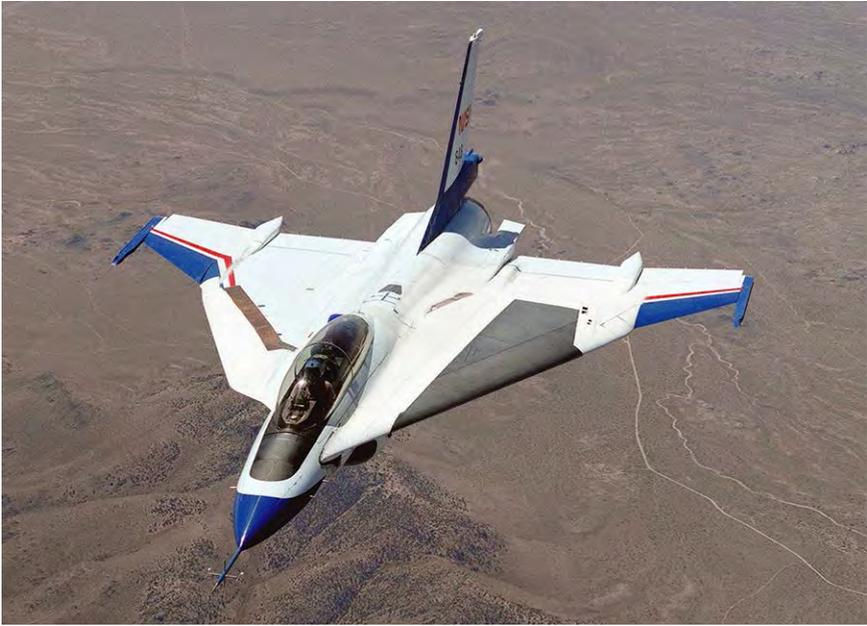
F-16XL-2 flying with a supersonic laminar flow control suction glove leading edge, April 1996. (NASA)
