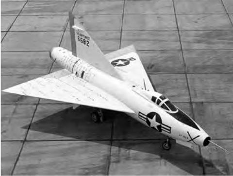
The Convair XF-92A Dart, progenitor of all American delta-wing aircraft, on the ramp of the NACA High-Speed Flight Research Station (now the Dryden Flight Research Center) in 1953. The wing and aft fuselage were tufted for flow visualization studies. Despite its “F” for “Fighter” designation, this was strictly a transonic research aircraft. (NASA)
