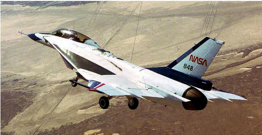
Research pilot Dana Purifoy flew the highly modified F-16XL-2 on its first flight with the asymmetrical wing configuration on October 13, 1995. Wingtip-mounted flutter excitation vanes are fitted on both wingtip missile launchers. (NASA)
