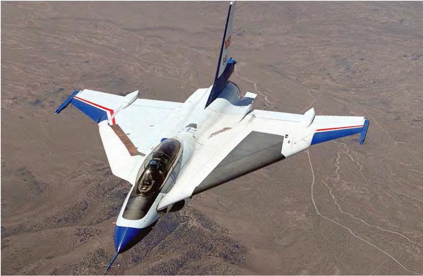
F-16XL-2 flying with a supersonic laminar flow control suction glove leading edge, April 1996. (NASA)
