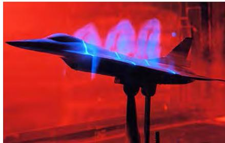
A  $\frac{1}{25}$ -scale F-16XL-1 model was tested in the Basic Aerodynamics Research Tunnel at NASA Langley Research Center in 1992. Laser light sheets illuminate the vortex flow field around the model. (NASA)
