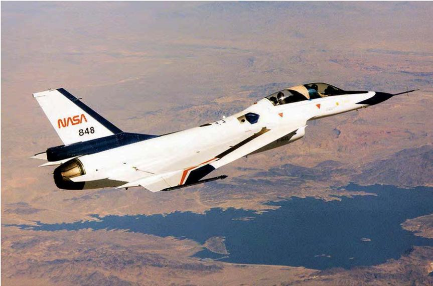
The turbocompressor exhaust duct exited the F-16XL-2 in the center-of-black region behind the rear cockpit. Note the special fairing mounted over the canopy frame to minimize shock wave formation. (NASA)
