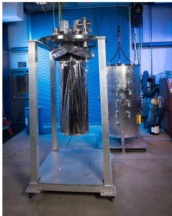
Figure 2: Calorimeter for testing multilayer insulation as low as 20 K.
