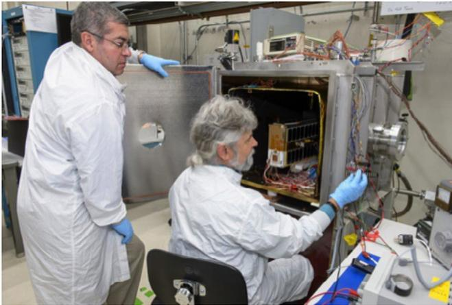
*NASA's first 6U nano-satellite, EcAMSAT, undergoes thermal vacuum power management (TVPM) testing at NASA Ames. The test simulates the thermal vacuum and power environment of space and is an element of the spacecraft's flight validation testing program.*
