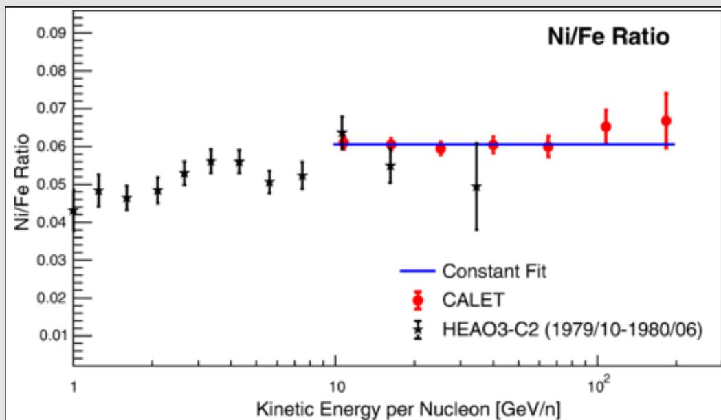
Figure 27. Nickel-to-iron ratio with statistical error bars. Constant fit demonstrates that the energy spectral shapes of the two nuclei are the same. Image adopted from Adriani, *Physical Review Letters*.
