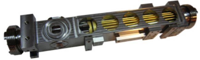
DSAC mercury ion trap housing with electric field trapping rods seen in the cut-outs. This is where DSAC interrogates and measures the mercury ion resonance that is used to discipline a quartz crystal clock.
