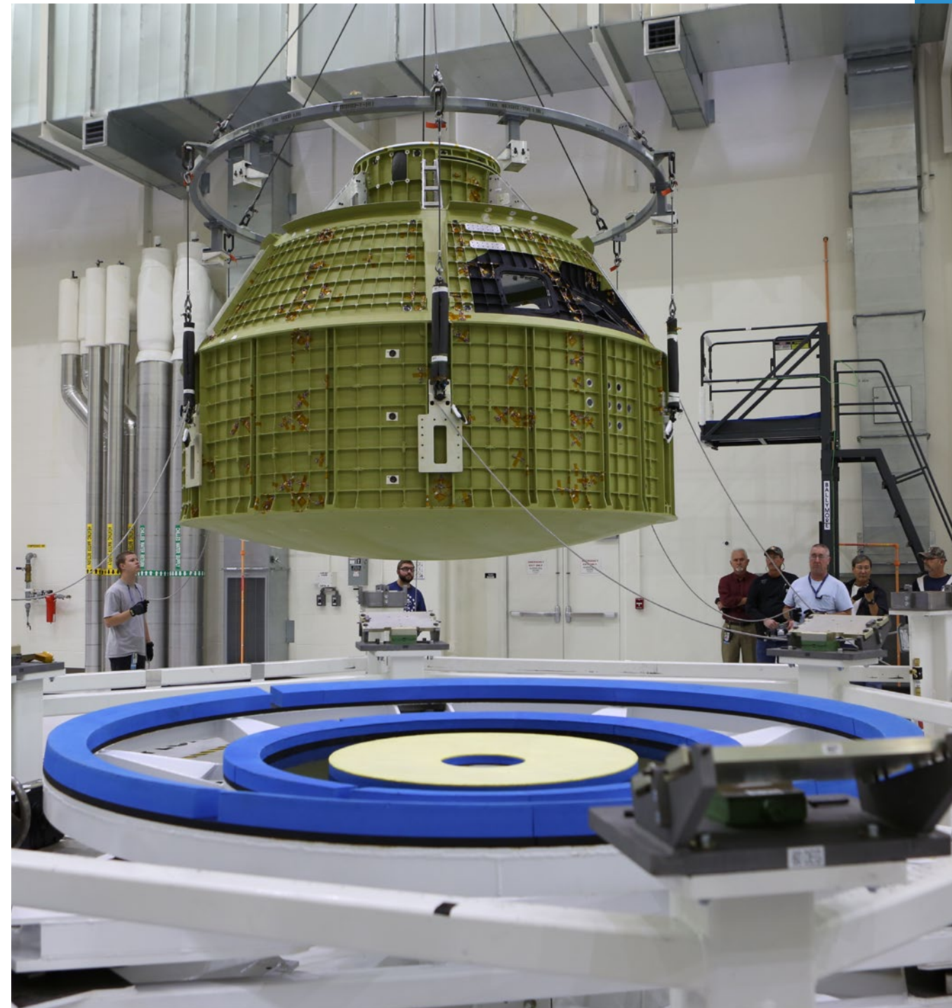
Lockheed Martin technicians monitor the progress as a crane lowers the Orion crew module structural test article (STA) toward a test tool called the birdcage inside the Neil Armstrong Operations and Checkout Building at Kennedy Space Center. The STA arrived aboard NASA's Super Guppy aircraft at the Shuttle Landing Facility operated by Space Florida. The test article will be secured on the birdcage for further testing. The Orion spacecraft will launch atop NASA's Space Launch System rocket on EM-1, its first deep space mission, in late 2018. Photo credit: NASA/Ben Smegelsky
