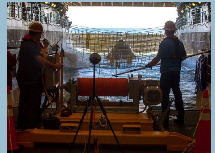
Winch team operators help guide a test version of the Orion crew module into the flooded well deck of the USS San Diego on Oct. 29 during Underway Recovery Test 5 in the Pacific Ocean off the coast of California. Photo credit: NASA/Bill White
