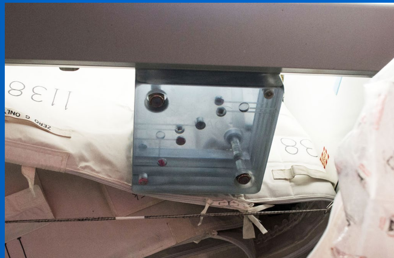
A sensor designed to detect radiation damage and materials fatigue now is at work aboard the International Space Station. The Detector for the Analysis of Solar Neutrons, or DANSON, was developed at the University of Nebraska. It was installed by NASA astronaut Shane Kimbrough shortly after its arrival aboard the Cygnus spacecraft. Such a device could generate electricity similar to a solar cell, but from neutrons instead of photons, to power NASA’s future deep space probes. Photo credit: NASA
