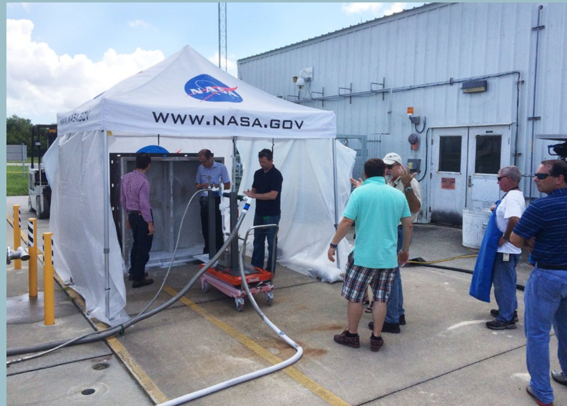
Members of Kennedy Space Center's Cryo Test Lab team set up the cold vapor test in which a newly developed nozzle created a wall of mist against a test panel loaded with sensors. Photo credit: NASA
