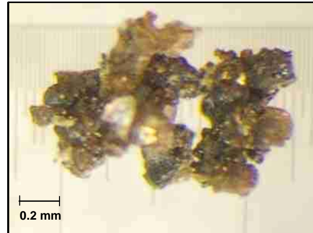
Agglutinate Simulant Particles Produced from JSC-1A Lunar Regolith Simulant
