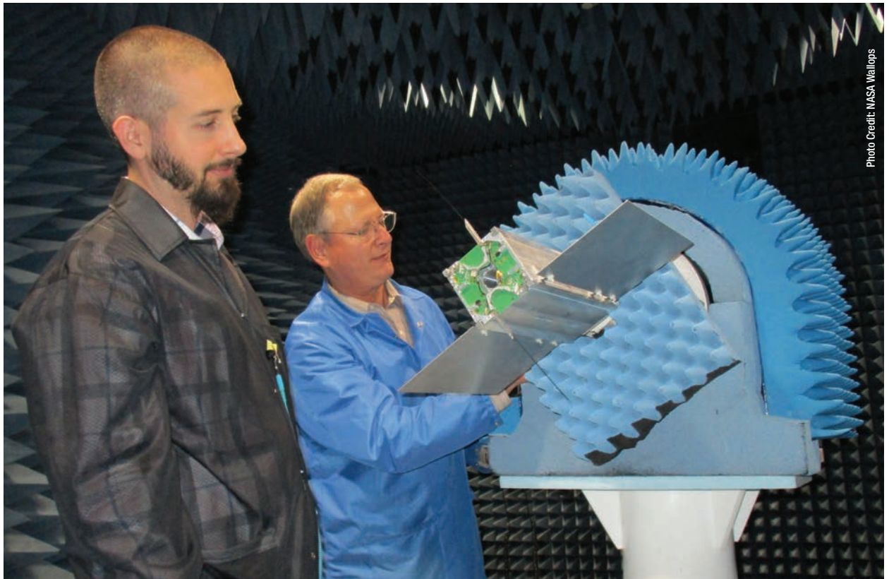
The Wallops Flight Facility's Brian S. Abresch (left) and Con Duer are shown here working on IceCube's UHF antenna. IceCube is designed to study ice clouds and test a commercial receiver for NASA's proposed Aerosol-Cloud-Ecosystems mission.
