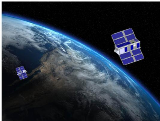
*The Tyvak Nano-Satellite Systems, Inc. designed CPOD 3U CubeSat incorporates a suite of RPOD sensors, high performance low power processors, modular flight software, and an advanced control system that includes a multi-thruster propulsion system.*
