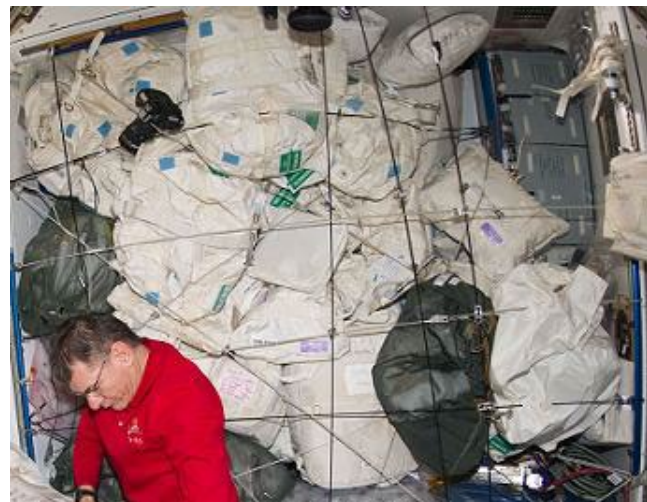
Restraints holding storage containers
