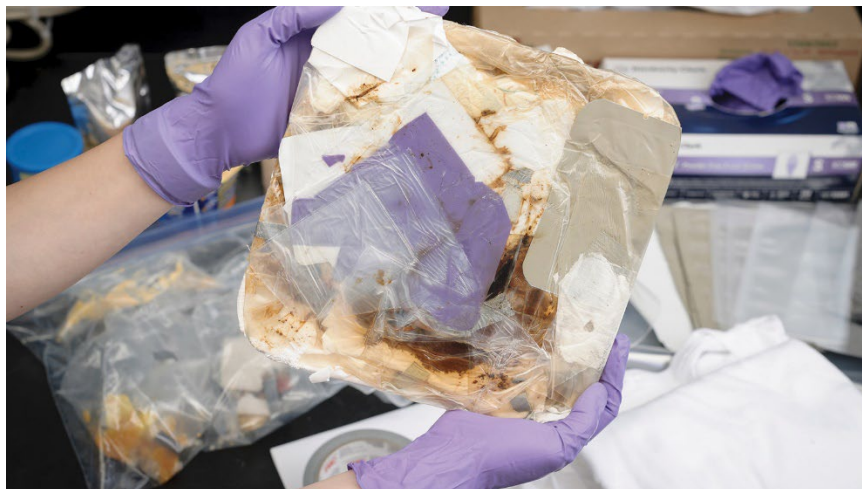
Trash melted into a tile using a heat melt compactor
