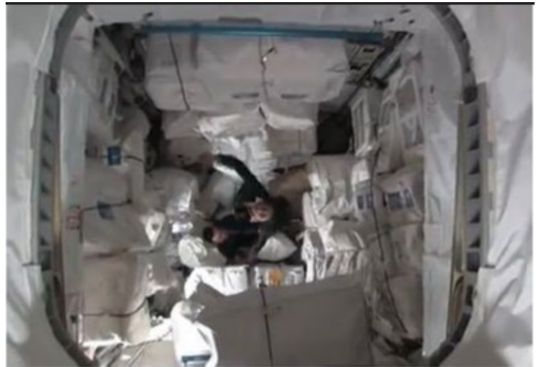
The Leonardo Permanent Multipurpose Module (PMM), installed in March 2011, is used for storage on the ISS.
