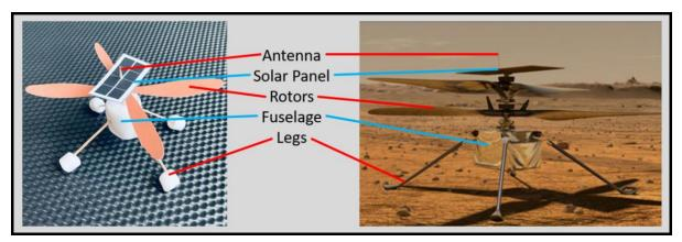
Figure 10. Comparison of your model to the actual Mars helicopter.
