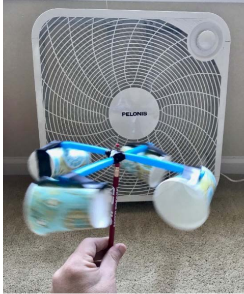
Figure 4. Place the anemometer in a stream of air to see it rotate
