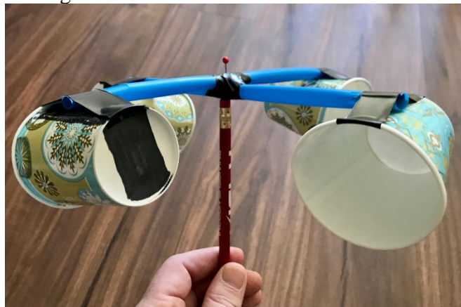
Figure 3. Attach the cups to the straws using a stapler
