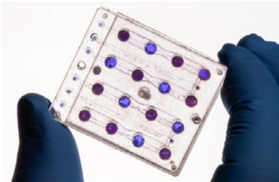
*BioSentinel's microfluidics card, designed at NASA Ames, will be used to study the impact of interplanetary space radiation on yeast. Once in orbit, the growth and metabolic activity of the yeast will be measured using a 3-color LED detection system and a metabolic indicator dye. Here, pink wells contain actively growing yeast cells that have turned the metabolic dye from blue to pink color.*
