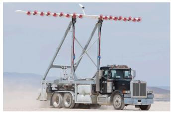
The integrated experimental testbed reached speeds of up to 73 mph in data collection to create the effect of a wind tunnel on the ground. (NASA Photo/Tom Tschida)
