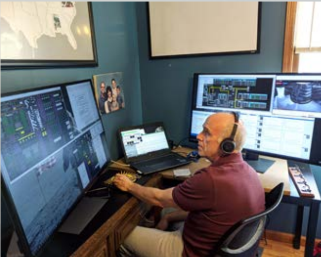
GRC-2021-CN-00029 Photo by Lenore Maul Maul operates the specialized console display software, which he helped develop to monitor live-streamed sensor measurements and status from the TVC subsystem.
