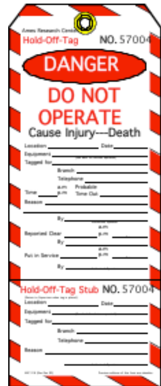
Figure 6.3: Master Danger Tag (Do Not Operate)
