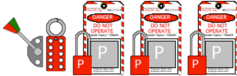
Figure 6.19: Single Group—Single Shift—Single Device
