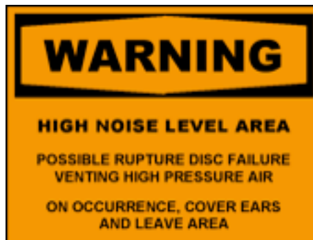
Figure 10.3: Warning Sign for Areas With Elevated Rupture Discs
