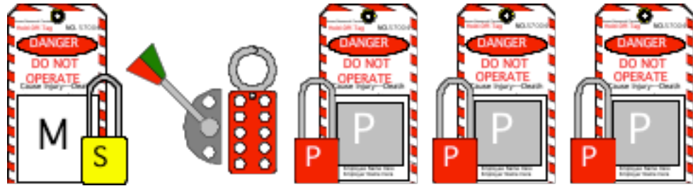
Figure 6.20: Single Group—Multiple Shifts—Single Device
