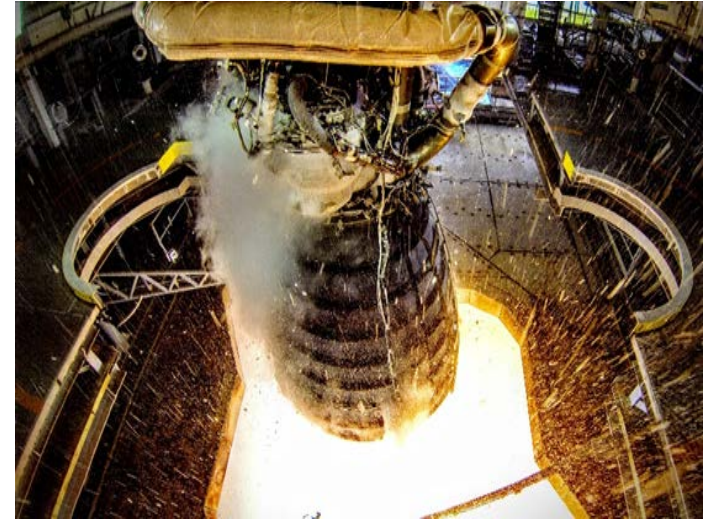
June 2015 hot fire of an RS-25D engine (modified version of the Space Shuttle Main Engine) on the A-1 Test Stand at the SSC. Four RS-25 engines will power SLS's core stage
