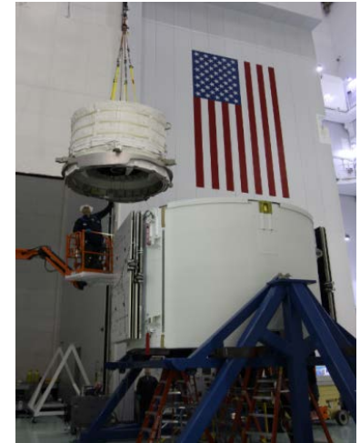
BEAM flight hardware being installed in SpaceX Dragon capsule's trunk
