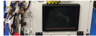
Space Automated Bioproduct Lab is an incubator used to conduct cell culture and other biological experiments
