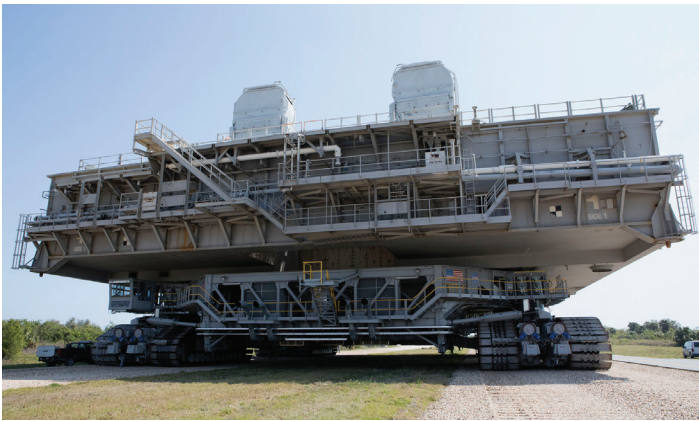
NASA's upgraded crawler-transporter 2 (CT-2), carrying mobile launcher platform 1, moves slowly along the crawlerway March 22, 2017, at Kennedy Space Center in Florida. The crawler's upgrades and modifications were monitored and tested under loaded conditions during its travel to the crawlerway Pad A/B split and back to the crawler yard to confirm it is ready to support the load of the mobile launcher carrying the Space Launch System with Orion atop for the first uncrewed test flight, Exploration Mission-1. Photo credit: NASA/Leif Heimbald
