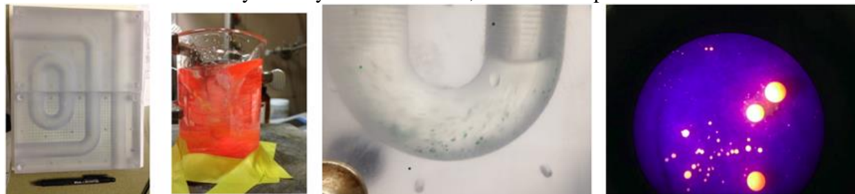
Figure 8. Far left: Machined flow channels. Left: Fluorescent particle synthesis. Right: Secondary flows visualized by green particles. Far Right: Newer fluorescent particles.
