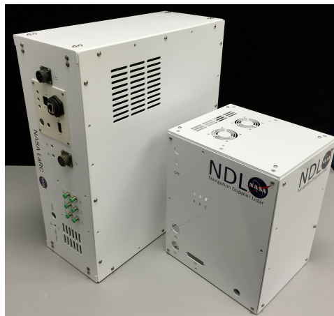
Figure 6. Miniaturized LiDAR chassis developed at NASA Langley in 2012 and 2016
