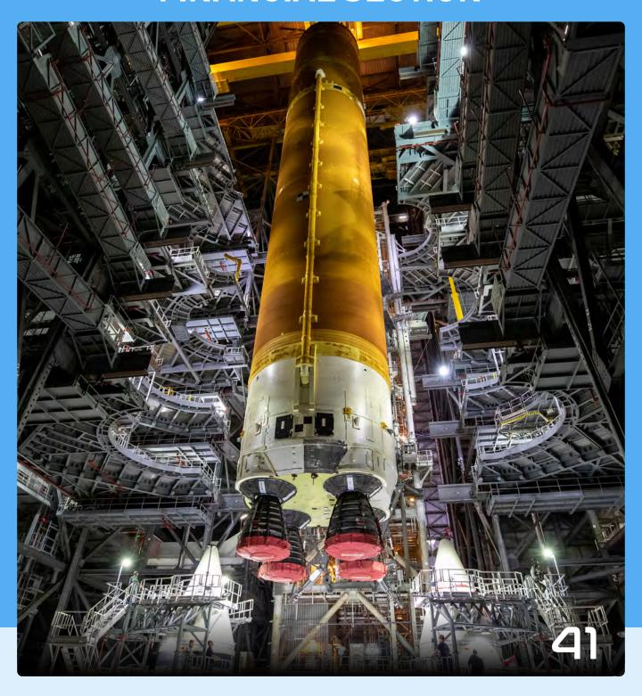
Teams with NASA's Exploration Ground Systems and contractor Jacobs prepare to lower the Space Launch System (SLS) core stage - the largest part of the rocket - onto the mobile launcher, in between the twin solid rocket boosters, inside High Bay 3 of the Vehicle Assembly Building at NASA's Kennedy Space Center in Florida on June 12, 2021.
