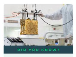
The growing list of "firsts" for Perseverance, NASA's newest six-wheeled robot on the Martian surface, includes converting some of the Red Planet's thin, carbon dioxide-rich atmosphere into oxygen. A toaster-size, experimental instrument aboard Perseverance called the Mars Oxygen In-Situ Resource Utilization Experiment (MOXIE) accomplished the task. The test took place April 20, the 60th Martian day, or sol, since the mission landed Feb. 18.
