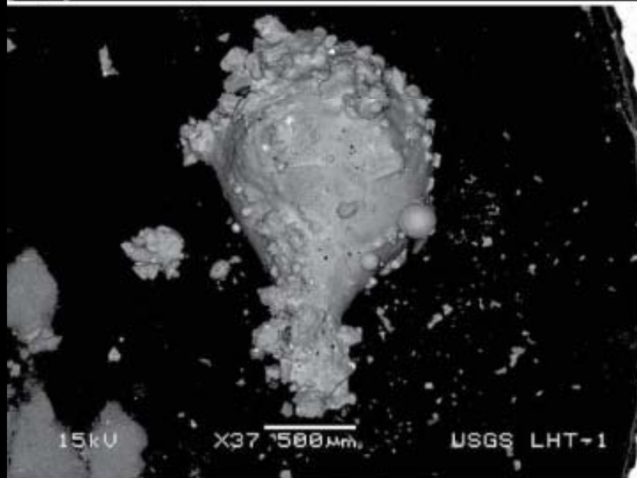
EXAMPLES OF LARGE PSEUDO-AGGLUTINATE PARTICLES FROM NU-LHT-1M PILOT
