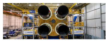
Four RS-25 engines attached to the core stage for Artemis I
