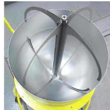
Vane-Type LAD integration into a tank
