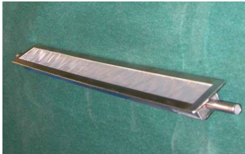
Breadboard screen-channel LAD for outflow testing
