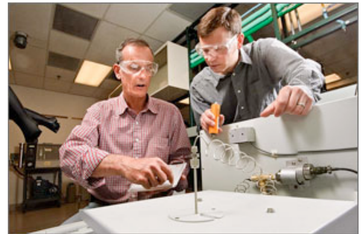
NASA engineer Eric Darcy, left, and NREL engineer Kandler Smith get ready to test lithium-ion batteries for how well they can combat rare but potentially catastrophic thermal runaways.
