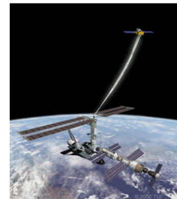
Electrodynamic Tether Propulsion Artist Concept of ISS Reboost
