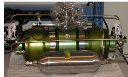
Pulse Tube Cryocooler for Oxygen Liquefaction
