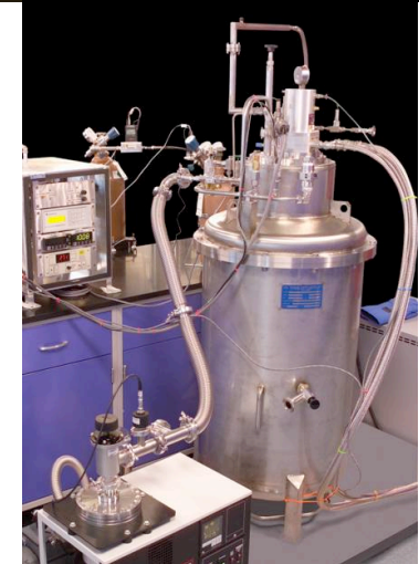
Integrated Refrigeration and Storage System
