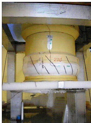
Aerogel Insulation used for External Tank LO2 Bellows Ice Elimination
