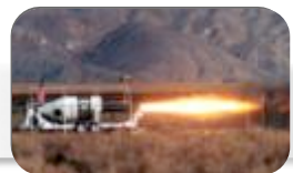
Spaceship One Hybrid Rocket Motor
