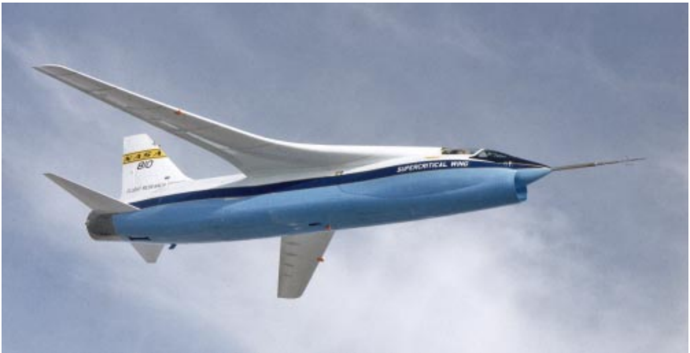
Supercritical wings add a graceful appearance to the modified NASA F-8 test aircraft.
