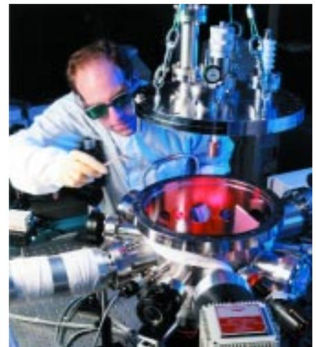
**Figure 26: NASA's Electrostatic Levitator is a unique tool—one of only a few in the world—that allows researchers to study molten materials, such as metals, alloys, and metallic glass, in a containerless environment here on Earth. The levitator keeps the sample in a perfectly spherical shape, making it easier for researchers to understand the physical phenomena that are taking place within the sample.**
