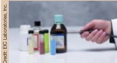
**Figure 25: Using a fiber-optic probe, the Raman spectrometer can analyze unknown substances through clear and semiclear glass and plastic packaging materials.**
