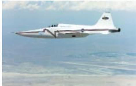
**Figure 22: Northrop-Grumman Corporation's modified U.S. Navy F-5E Shaped Sonic Boom Demonstration Aircraft.**
