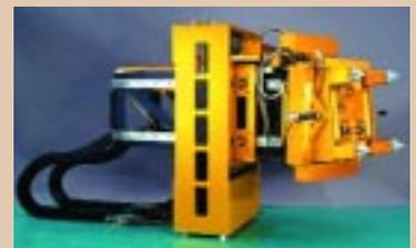
**Figure 21: The umbilical system is one of the most advanced fueling systems currently available because it decreases the need for human intervention during potentially dangerous fueling operations.**
