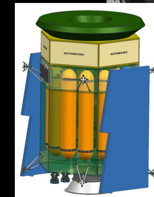
Propellant Feed System and Storage Tanks
