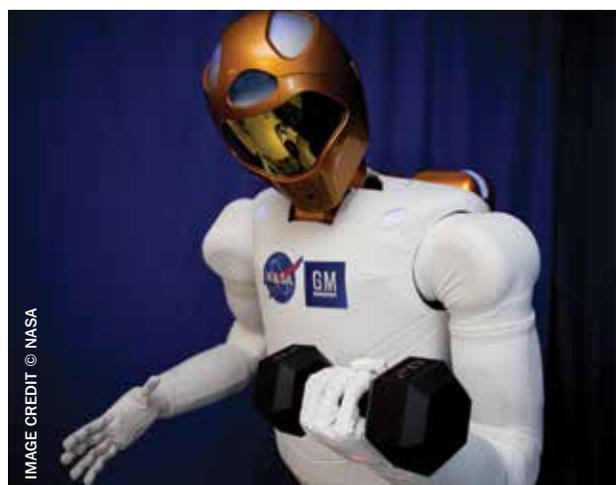
R2, the first humanoid robot created by GM / NASA was sent to the space station with the intention of eventually taking over tasks too dangerous or mundane for astronauts
