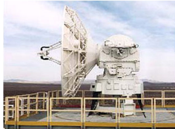
Figure 2: WATR instrumentation radar
