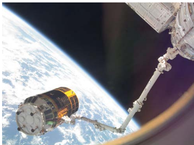
Figure 1: Canadarm2 with a Japanese HTV in its grasp
