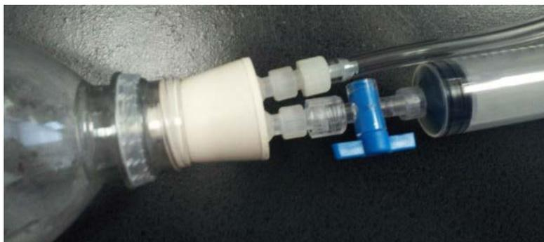
Figure 1: Bottle with pressure/fill cap
