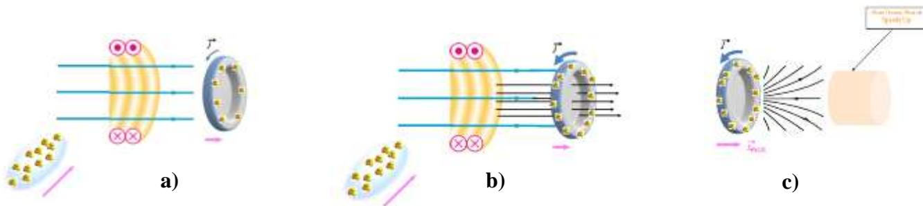
**Figure 3.2.2-2 - Formation of the “magnetic piston”. a) Formation of current layer in a cylindrical shape b) As more particles are collected the current in the layer increases that, in turn, increases the magnetic field. c) The moving layer approaches and pushes the bunch.**
