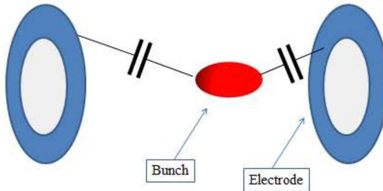
**Figure 3.4.3-1 – Schematic of the capacitive coupling of the bunch in between two TWDEC electrodes**
