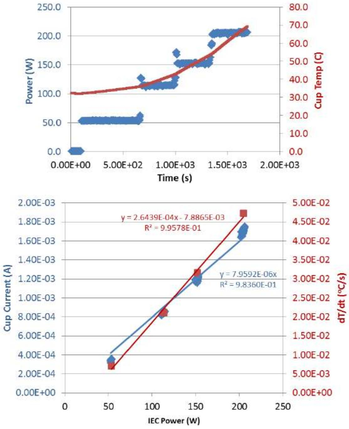
Figure 3.5.2-3 Thermal data from the Faraday cup
