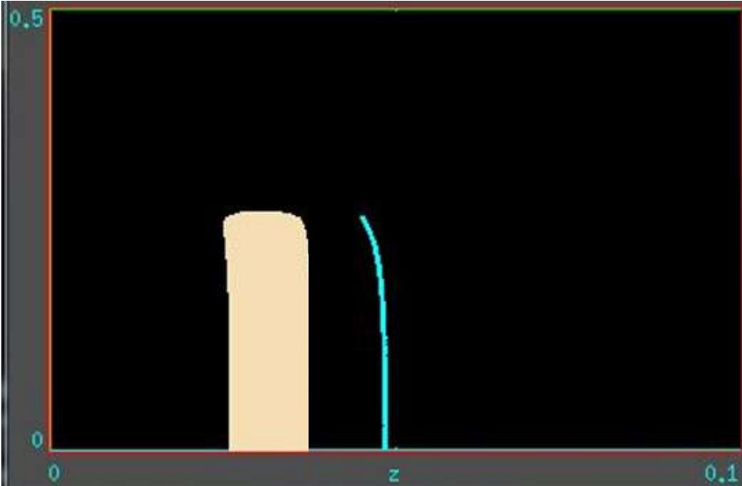
*Figure 3.3.2-4 –Further evolution in time of the bunch interaction: the fast bunch has reversed its velocity. The radial expansion is also now noticeable (there is no confining magnetic field). The axial (z-) expansion is more pronounced for the slow bunch as it has higher density.*
