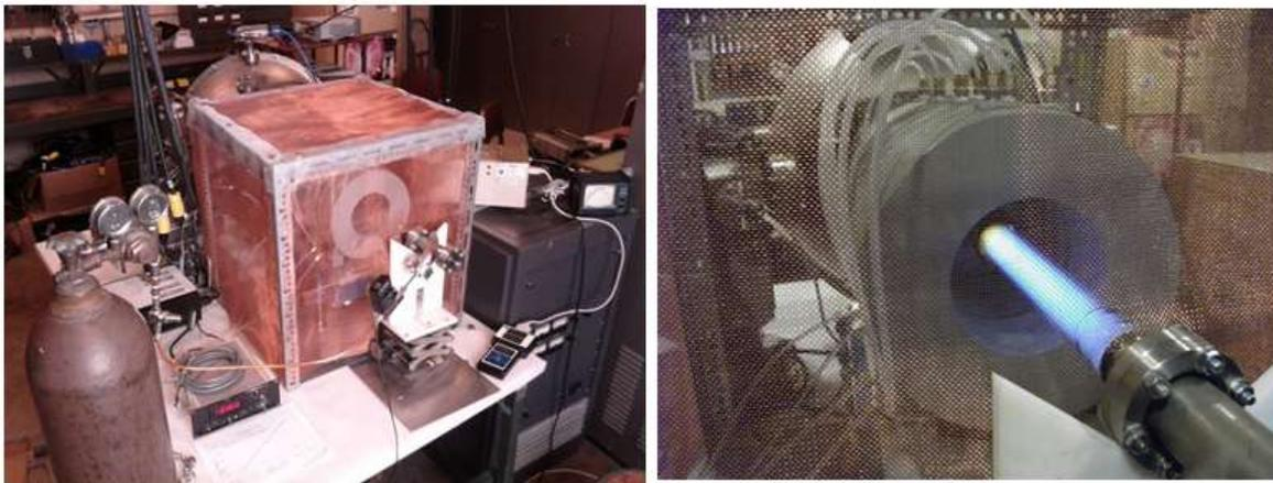
*Figure 3.5.1-2. IEC Device at UIUC: plasma from a 300 W Helicon source*
