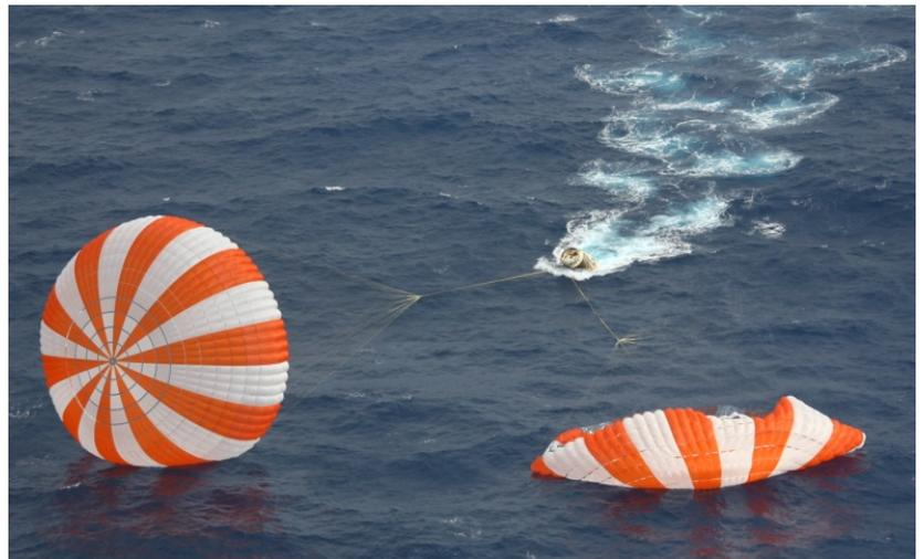
SpaceX will use a 100-foot boat equipped with an A-frame and an articulating crane, a 90-foot crew boat for telemetry operations, and two 24-foot rigid-hull inflatable boats to perform recovery operations. On board will be approximately a dozen SpaceX engineers and technicians as well as a four-person dive team. Once Dragon splashes down, the team will first secure the vehicle and then place it on deck for the journey back to shore.
