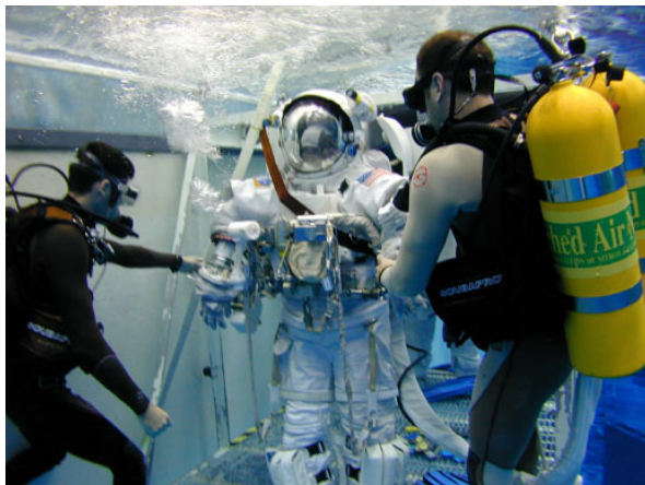
Figure 1: Astronaut Barbara Morgan participating in an underwater simulation of extravehicular activity (EVA) with diver assistance at the NBL
