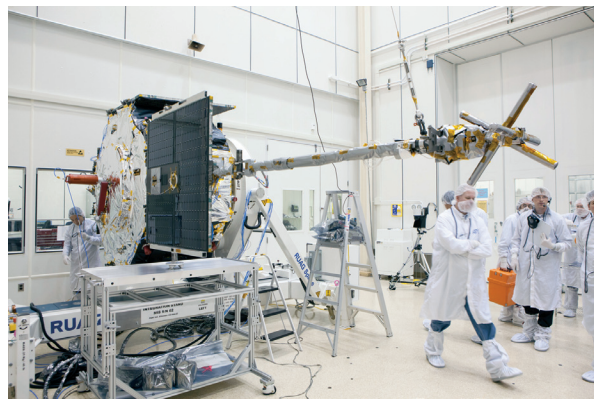
Above left: The EMFISIS tri-axial Magnetic Search Coil (MSC) magnetometer boom, shown stowed on the deployed solar array of spacecraft A; right, the MSC boom shown after deployment on spacecraft A
