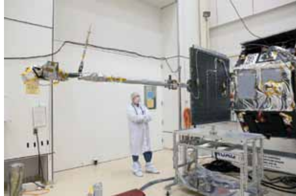
Above left: The EMFISIS tri-axial Fluxgate Magnetometer (MAG) boom, shown stowed on the deployed solar array of spacecraft A; right, the MAG boom shown after deployment on spacecraft A
