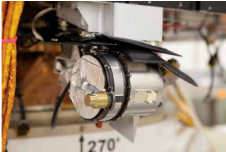
Above: The Radiation Belt Storm Probes Ion Composition Experiment (RBSPICE) installed on spacecraft B.
