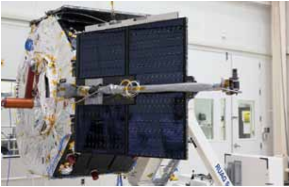
Above left: The EMFISIS tri-axial Fluxgate Magnetometer (MAG) boom, shown stowed on the deployed solar array of spacecraft A; right, the MAG boom shown after deployment on spacecraft A
