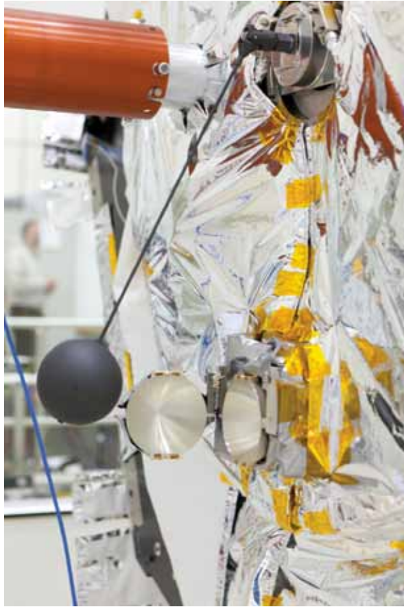
Above: The top sphere and antenna from the EFW axial boom of spacecraft A.
