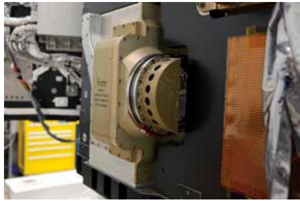
Above left: The Helium Oxygen Proton Electron (HOPE) instrument for spacecraft A; right, HOPE installed on spacecraft B
