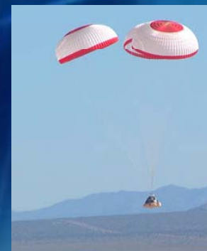
Successful parachute drop test accomplished during CCDev2
