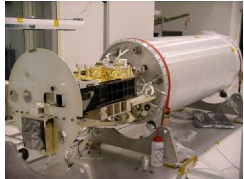
The payload was built in 2006 to accommodate the SDO EVE MEGS and ESP channels. This rebuild included larger rocket skins (22 inch diameter instead of 17 inch diameter). The NASA telemetry (TM) subsystem was updated to a 10 Mbps TM system to handle the higher volume of data from the CCDs on MEGS.
